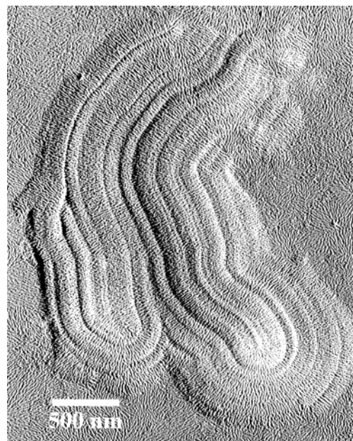
Figure 11. TEM morphology of the self-assembled columns after PE SLD.
